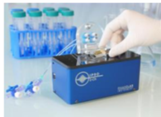
Figure 3: "IPSOLab", a 2 channels compact SPR.
